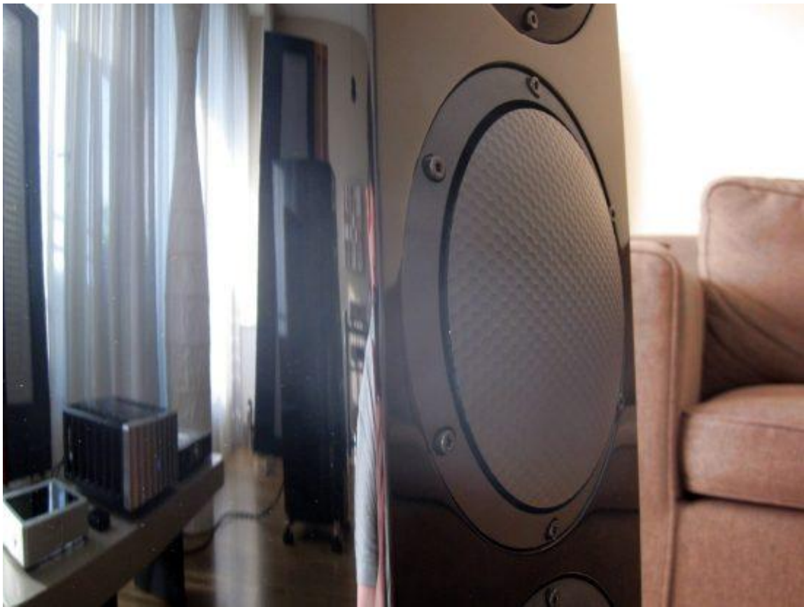
The woofers utilise an aluminium honeycomb sandwich and protrude outward, to make for a very nice, clean look.
